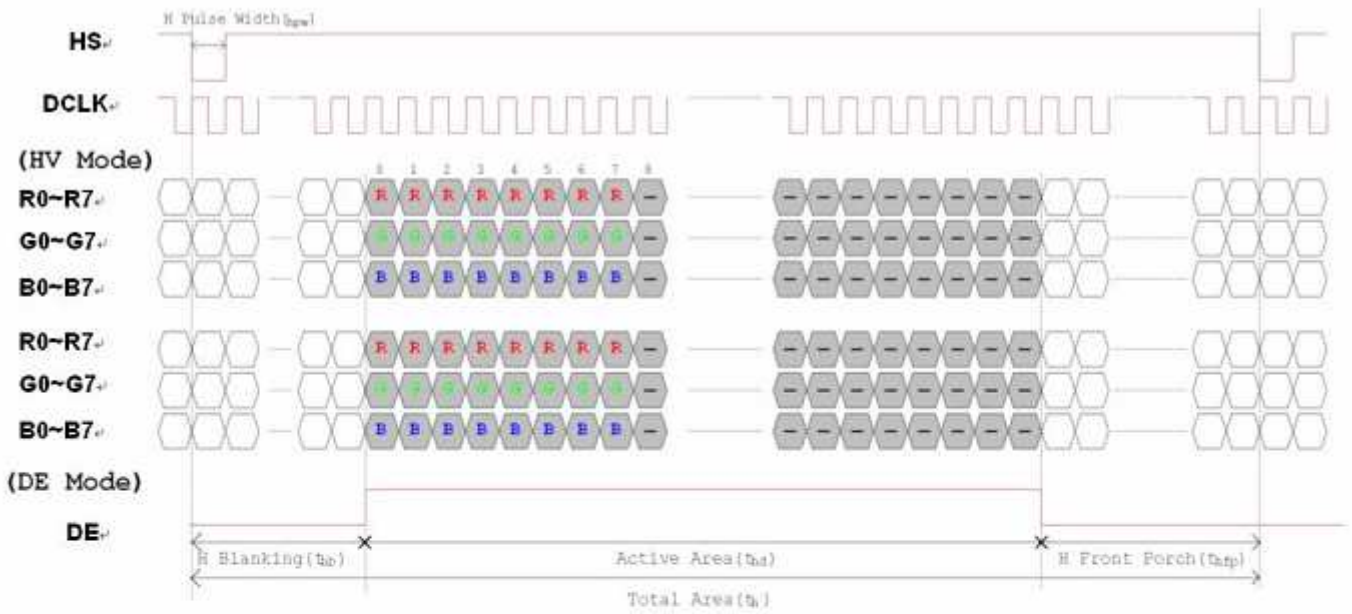
Figure 3. 1 Horizontal input timing diagram.
